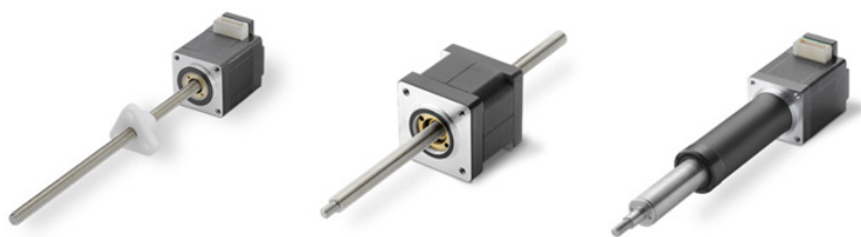
Figure 1 The three types of SMLAs (left to right: rotating screw, rotating nut and telescoping) feature unique mechanics that make them ideal for varying applications (all images courtesy of Thomson Industries).
