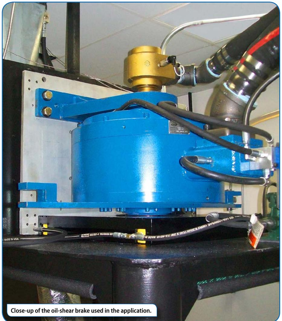
Close-up of the oil-shear brake used in the application.
