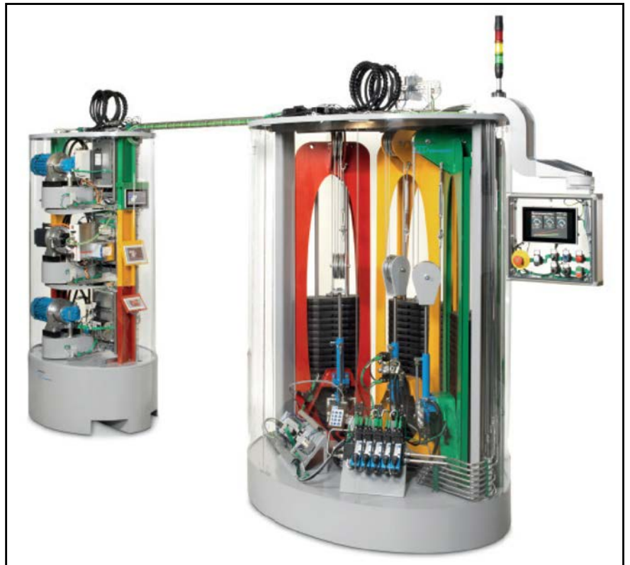
Figure 1 The machine model jointly developed by Eaton and solution partner ATP Hydraulik is based on three different drive concepts and demonstrates potential energy efficiency gains. (All images courtesy Eaton Corp.)
