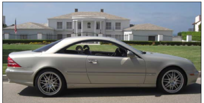
Figure 2 Shows a luxury vehicle with longitudinally oriented combustion engine and a driven rear axle. This concept is used by all automobile manufacturers worldwide on luxury-class vehicles that feature one driven axle.
