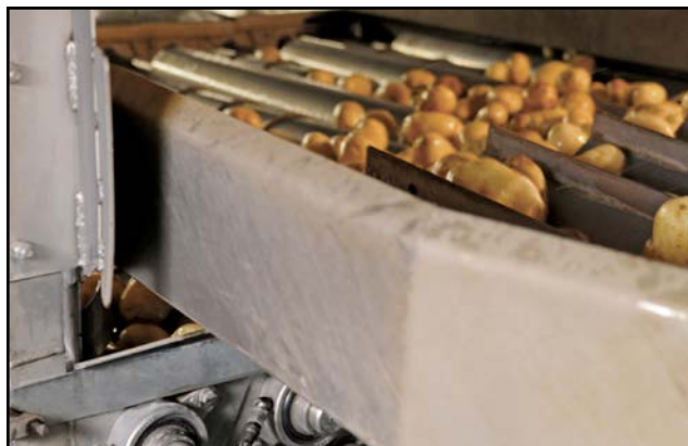
Bearing failures on this roll sizer machine were causing significant downtime at a Lamb Weston potato products plant. After installing a stainless steel mounted ball bearing with a superior sealing system that retains lubrication and prevents washout in wet environments, this machine went from being the least reliable to the most reliable.
