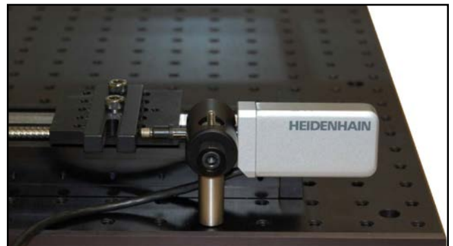
Figure 6 Setup for measuring X error.
