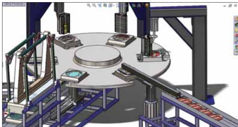
Solidworks can analyze mechanical systems by calculating actuator forces, motor torques, etc. (courtesy of Dassault).
