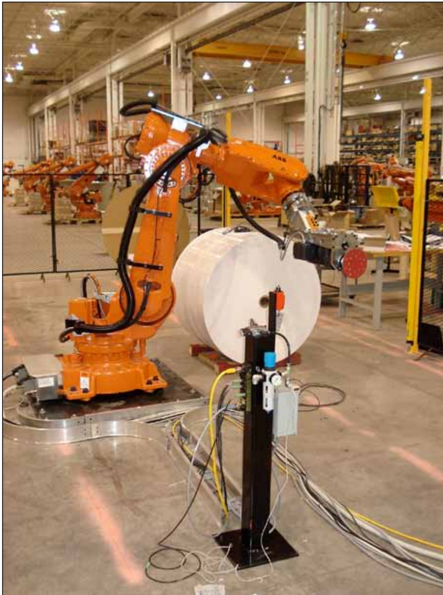
The ABB IRB 6620 is a flexible six-axis robot with a compact design.
