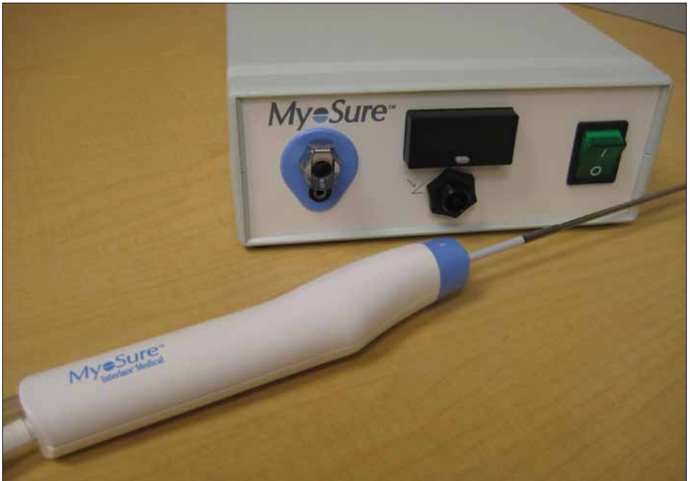
The MyoSure Tissue Removal System was upgraded with Maxon's RE40 motor and EPOS controller.
