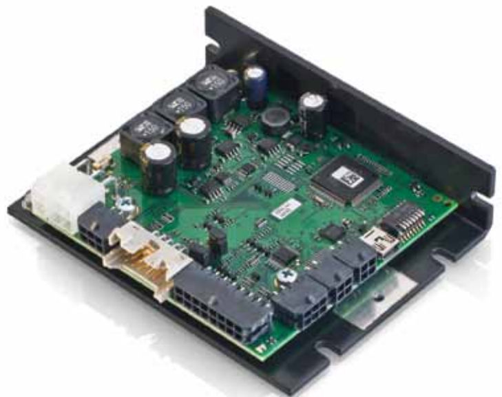
The EPOS controller uses simple logic and control functions for monitoring the motor.
