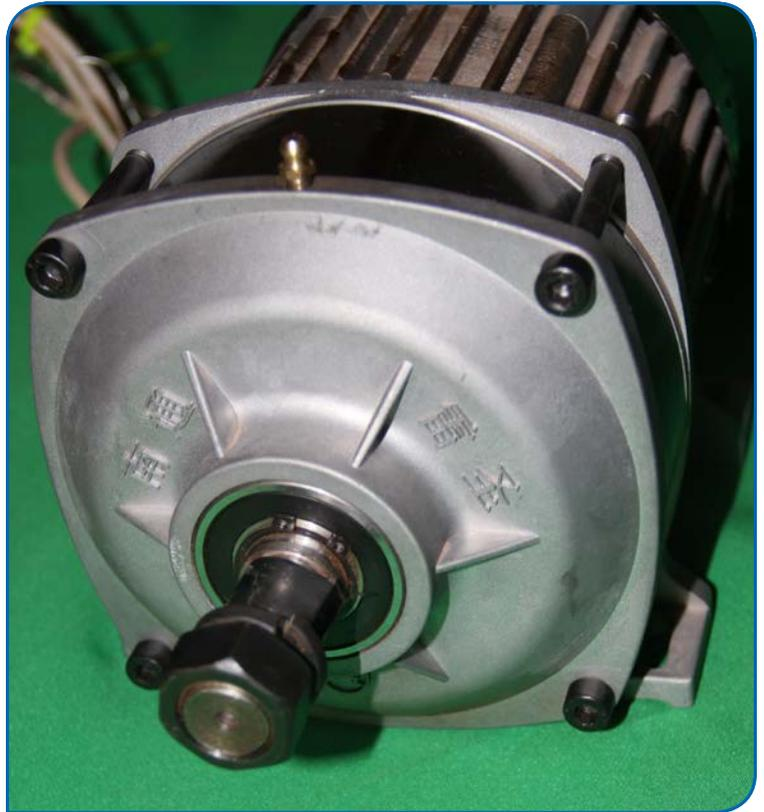
This Chinese-made gear motor is a switched reluctance traction motor with internal plastic gear (Photo courtesy Rocky Mountain Technologies).
