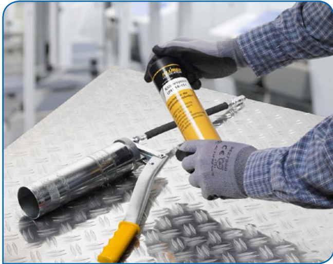
Figure 6 Grease guns can be filled manually or can be used in conjunction with a grease cartridge. Grease cartridges can allow for simple, clean relubrication with little waste.
