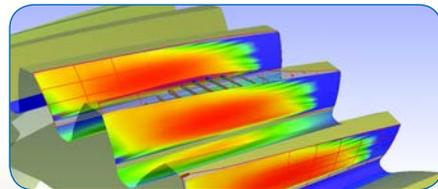
problem is caused by the response of the casings or mountings to the excitation coming from the gear mesh. This explains why gear noise can be so difficult to eradicate by changes to the gear geometry; i.e.—the real culprit is a system-level interaction—not a component-level “defect.”
