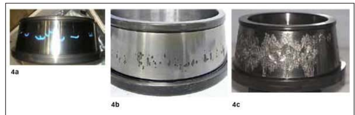
Figure 4 Failure appearance: a) straight cracks; b) straight cracks and small spalls; and c) spalls.
