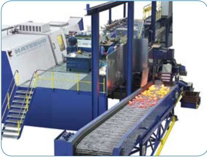
Figure 2 Hatebur amp 70 high-speed forge general bearing state-of-the-art grinding lines.
