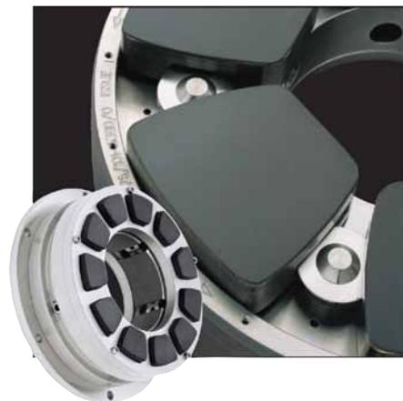
include highly customized journal—or combined journal and thrust—units designed to interface with an external pressurized oil system. Proven arrangements can be fitted with an external casing or engineered to interface with the customer’s own housing. The extent of supply, including hydraulic jacking systems, can be varied to suit application requirements and customer specifications.
