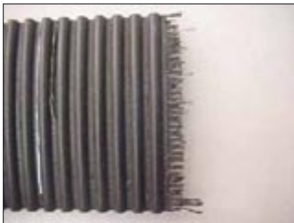
Figure 20—Crimp failure due to debris.
