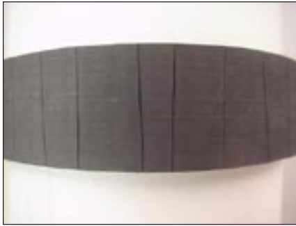
Figure 17—Cracking from high-temperature operation, rubber.
