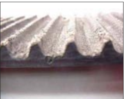
Figure 9—Excessive tooth wear.
