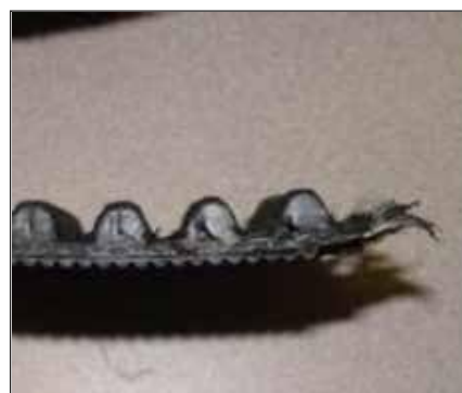
Figure 5—Tooth root crack propagation.
