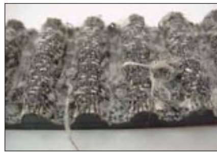
Figure 12—Extreme tooth wear from worn sprockets.
