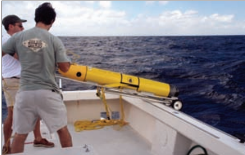
WHOI scientist Dave Fratantoni and postdoctoral scholar Benjamin Hodges prepare to lower the thermal glider into the ocean in December 2007.
