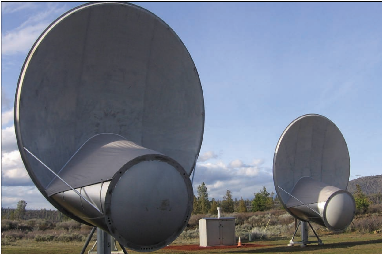
Figure 1—View of two antenna elements of the Allen Telescope Array at Hat Creek.
