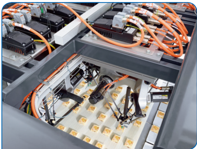
Bosch Rexroth's IndraDrive Mi provides cabinet-free drive technology.
