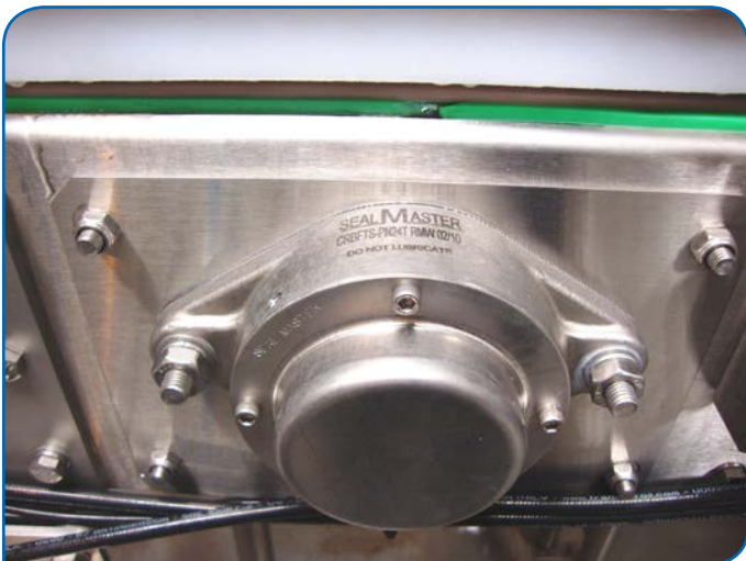
The added protection of end caps and backside shields can significantly prolong the life of a sealed bearing in clean-in-place and steam-in-place applications.
