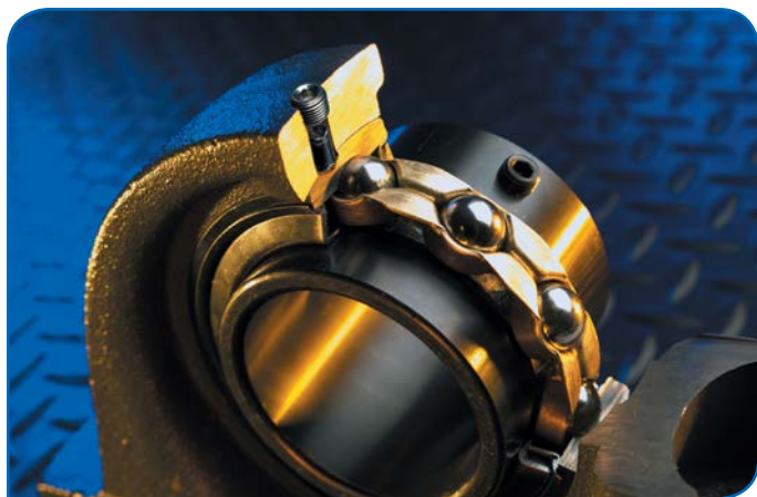
A retainer that rides on the outer ring land surface allows the balls to freely rotate in the cage pockets with a proper film of lube. A retainer that rides on the balls prevents the balls from rotating freely, so with every rotation grease is wiped from the ball.
