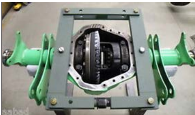
Photo 3 Housing spreader tool to aid in installing differential bearings in a rear axle. When the housing is released, the bearings will be preloaded and the remaining housing tension will aid in maintaining preload as the bearings wear.
