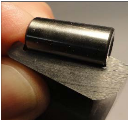
Photo 1 TRB cross-section highlighting rib/roller interface.
