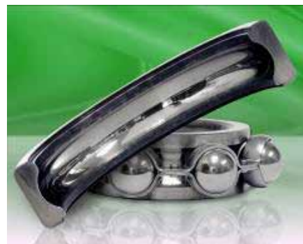
Figure 3—Taken from a failed motor, the fluted bearing race wall (left) resulted from VFD-induced bearing currents. Protected by an Aegis SGR bearing protection ring, the race on the right is undamaged.
