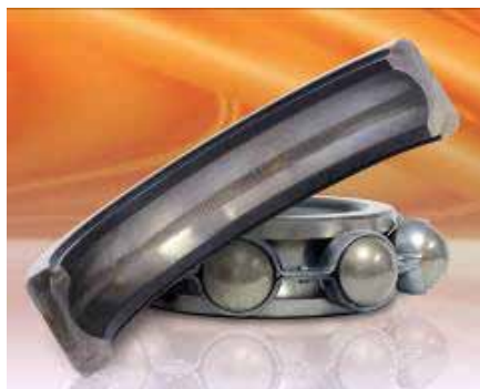
Figure 3—Taken from a failed motor, the fluted bearing race wall (left) resulted from VFD-induced bearing currents. Protected by an Aegis SGR bearing protection ring, the race on the right is undamaged.
