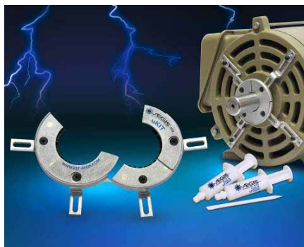
Figure 7—The Aegis SGR bearing protection ring is available for any size NEMA or IEC motor. It can be factory-installed inside new motors, as with the Baldor Super-E NEMA premium motor (left) or quickly and easily retrofitted—even in the field—using conductive epoxy (right). A new Split uKIT simplifies and speeds mounting of the ring on motors with shaft shoulders, slingers or other end-bell protrusions.
