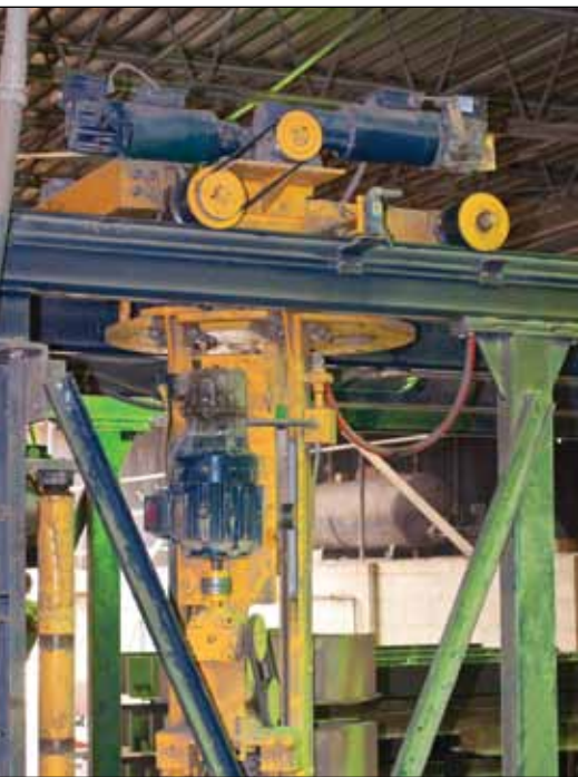
The motor on a clutch-brake assembly runs constantly, eliminating the starting and stopping to allow larger motor life.
