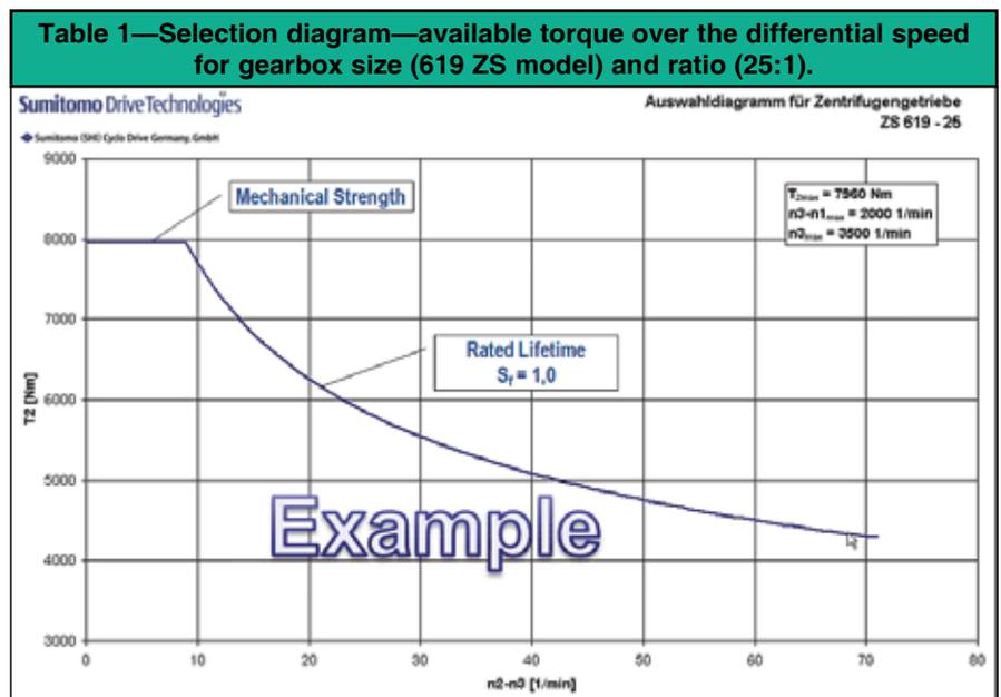
factor = 1.0) in that it has a B10 life of 8,000 hours. If we continuously run the machine at 40 rpm and a little over 5,000 Nm, then we have a rated life of approximately 8,000 hours. This is the philosophy behind selecting the correct product.
