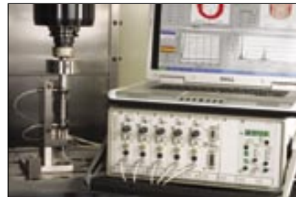
Figure 3—The spindle for a CNC vertical machining center with variable speed, AC motor and angular contact ball bearing spindle. The five probes are configured in a stiff nest for measuring motions of a two-sphere target rotating in the spindle. The probes will measure the total of bearing error motion, structural error motion, target eccentricity and target non-roundness. Boring a hole with this spindle would be an example of a rotating sensitive direction (courtesy of Dr. Eric R. Marsh).
