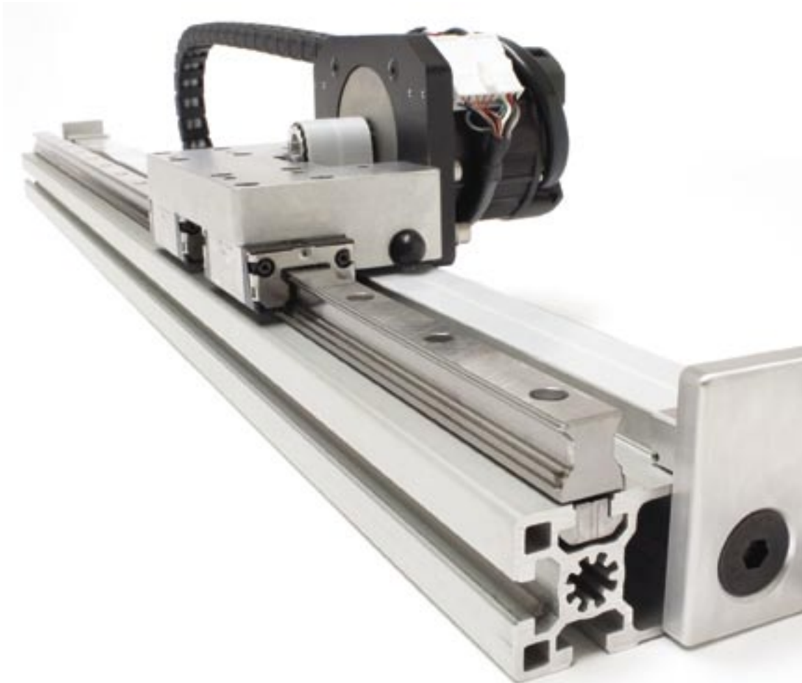
The ServoBelt combines Bosch Rexroth ball rail guides and aluminum framing with a belt-driven carriage, providing the speed and accuracy of a linear motor at a value comparable to belt-driven actuators (courtesy of Bosch Rexroth).
