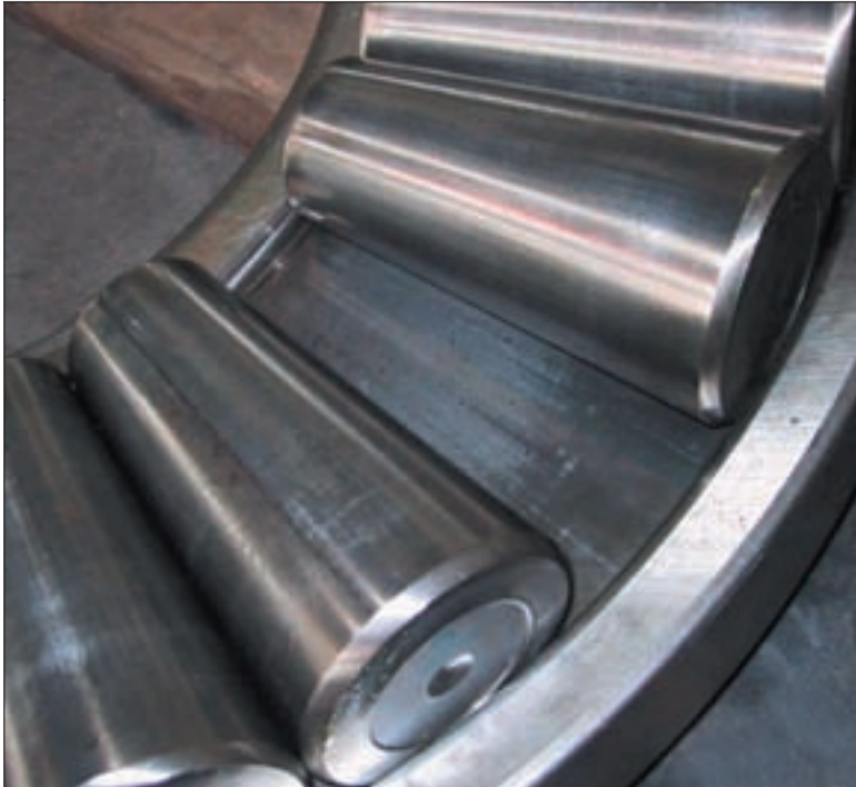
Thrust roller bearings and outer race before the bearing repair process.
