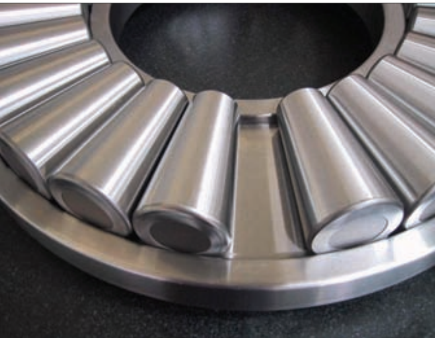
Thrust roller bearings and outer race after the bearing repair process.
