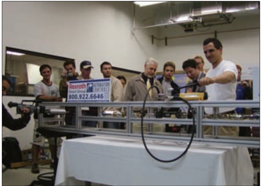
The strong tether competition tests the tensile strength of proposed elevator tethers.
