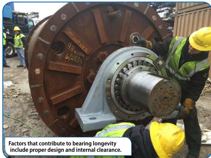
Factors that contribute to bearing longevity include proper design and internal clearance.
