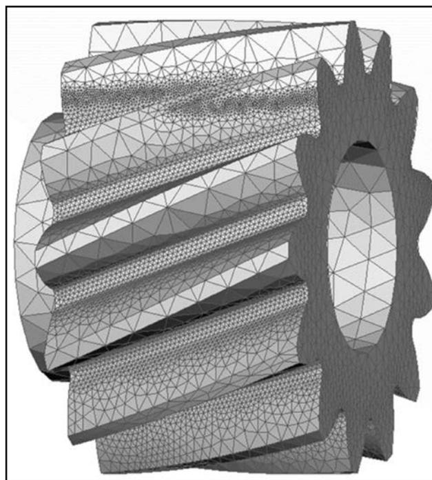
Figure 6 3-D FE mesh of the sun gear.
