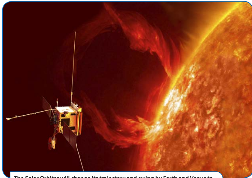
The Solar Orbiter will change its trajectory and swing by Earth and Venus to reduce its distance from the sun to only 45 million kilometers. Temperatures rise up to 520°C under the ceaseless pounding by solar radiation. All other sides are surrounded by the eternal cold of outer space making for an incredibly challenging environment (photo credit 2016 ESA – C. Carreau).
