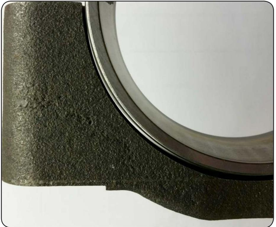
Figure 2 Bearing cap after machining and removal.
