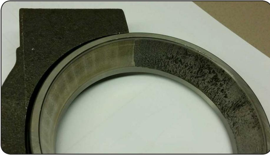
Figure 3 Bearing cup spalling at the cap interface.
