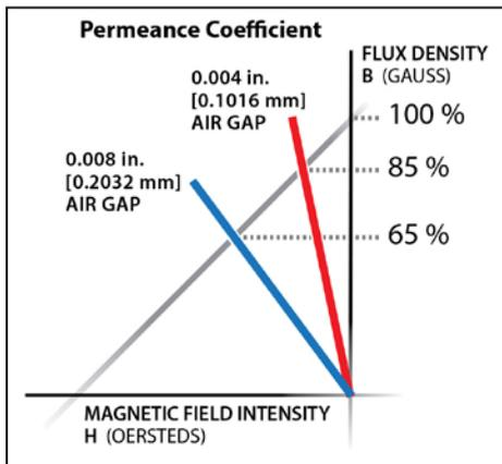
Figure 4 Effect of air gap on motor efficiency and performance.
