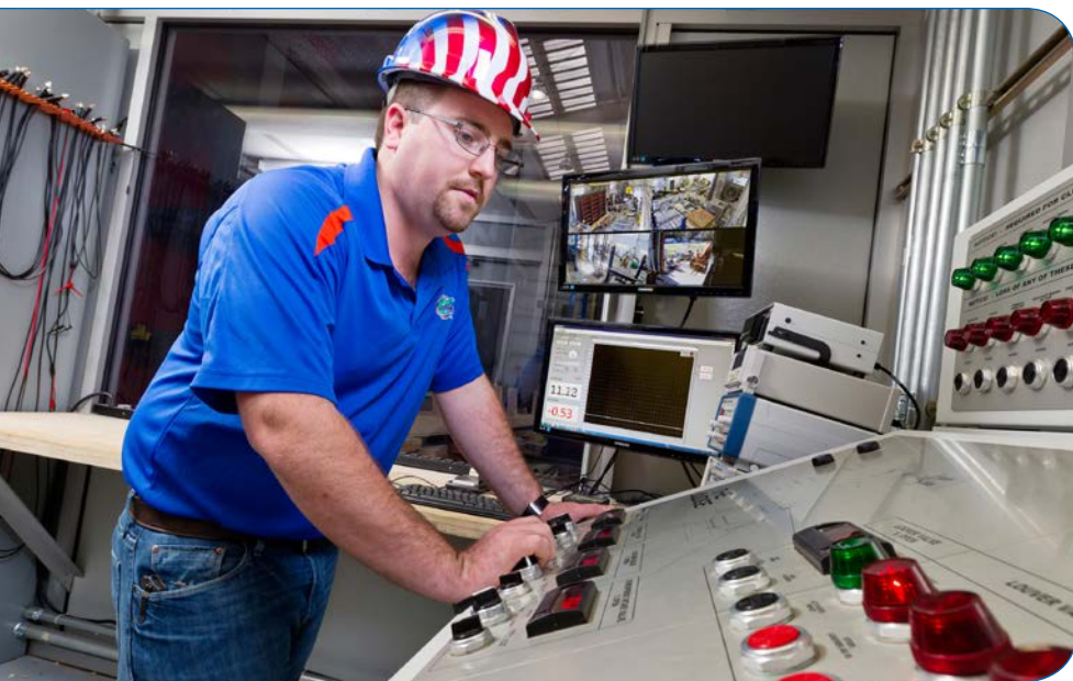
J. Alex Esposito, M.E., E.I.T, lab manager, Powell Family Structures and Material Lab at the simulator’s analog control panel designed by Henry Upjohn. Monitors and equipment for digital test data capture are seen in background.
