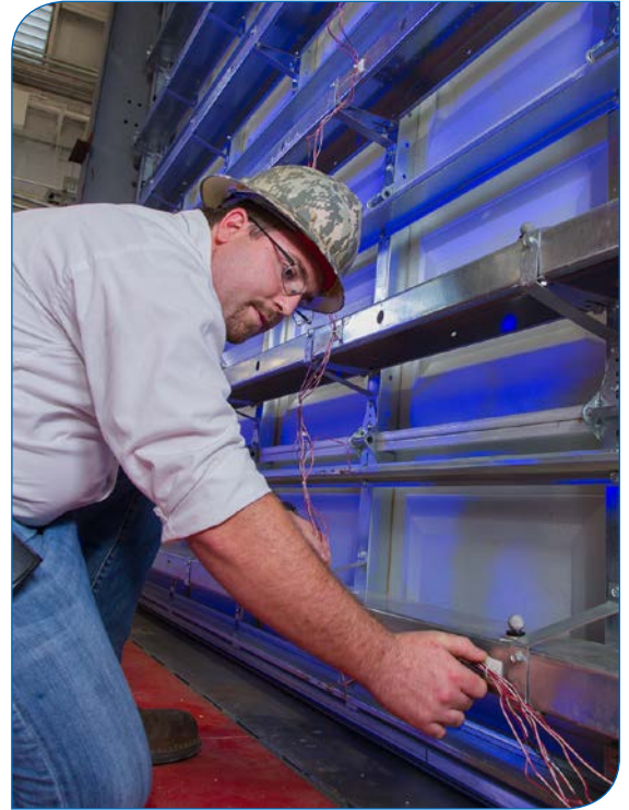
Setting strain gauges on subject door prior to testing.
