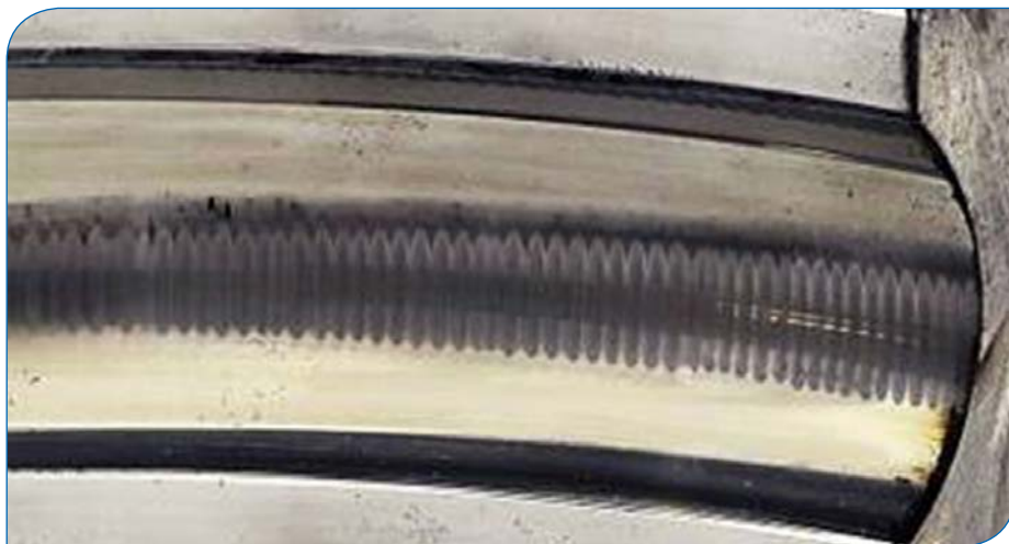
Figure 2 In a process called fluting, pits form washboard-like ridges on a bearing race wall — ridges that cause still more noise and vibration and accelerate bearing failure.
