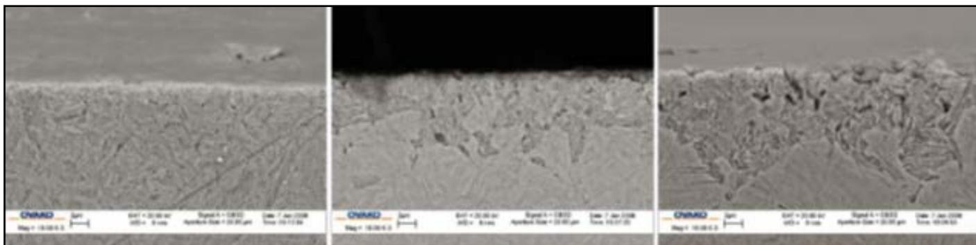
Figure 7 SEM micrographs of the surface microstructure — 2 percent nital-etched.
