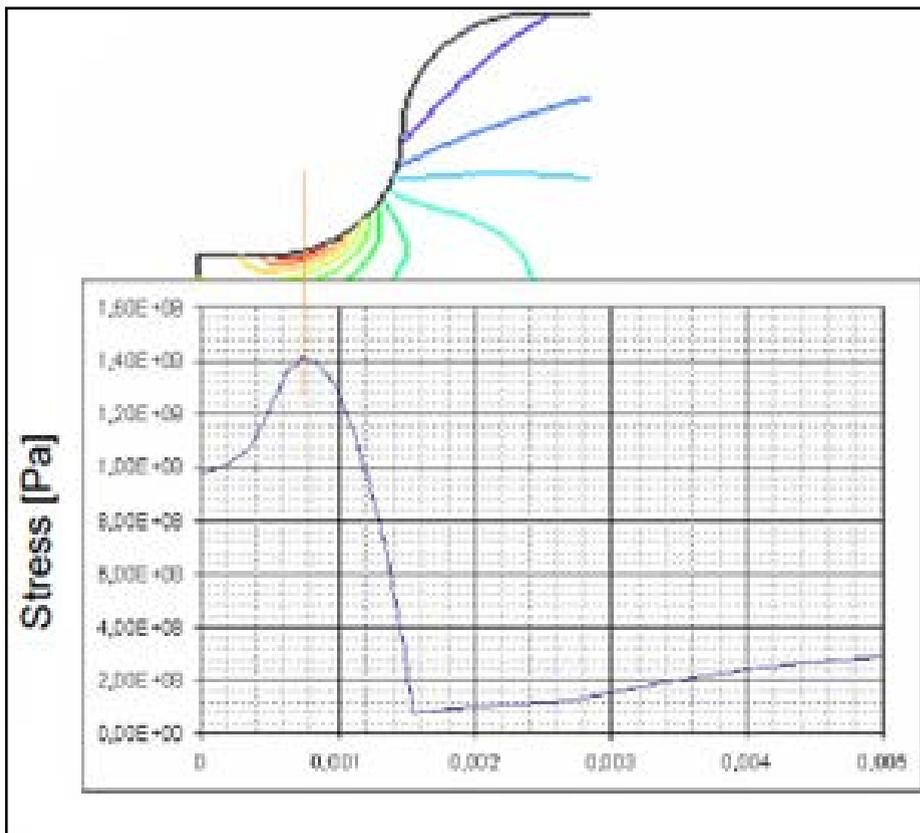
Figure 9 FEM calculation of highest-stressed region.
