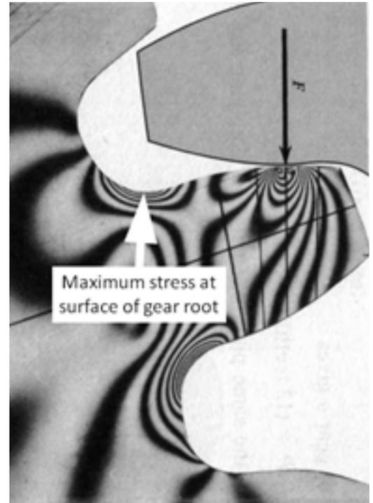
Figure 1 Failure initiation points.
