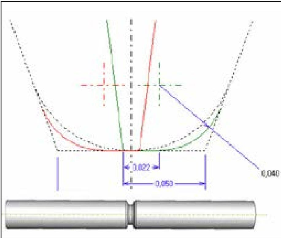
Figure 8 Notched test sample and gear root geometry.
