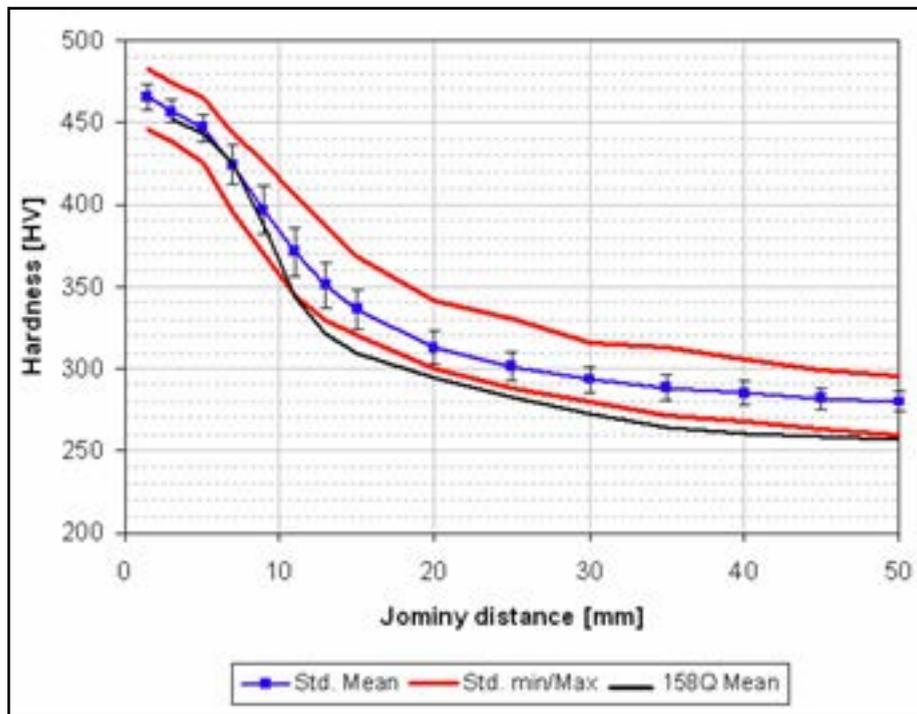
Figure 4 Jominy hardenability: measured hardenability of grade 158Q compared to existing grade.
