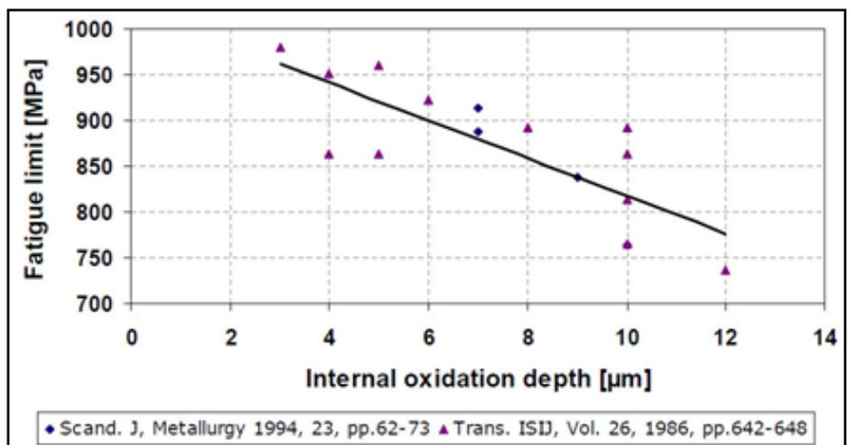
Figure 2 Internal oxidation and fatigue limit: literature indicated a potential gain of 100 MPa in the fatigue limit if the internal oxidation is restricted to 2  $\mu\text{m}$  maximum.
