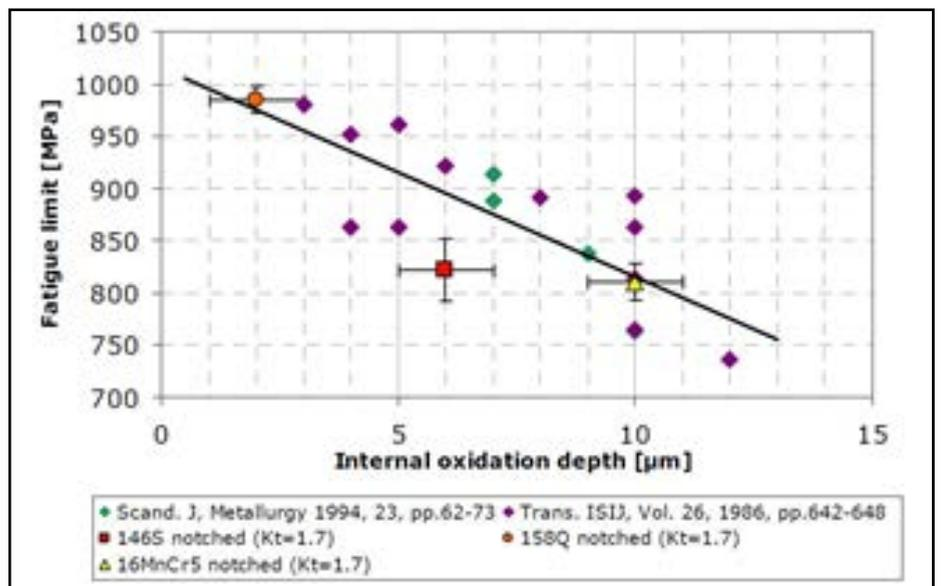
Figure 12 Effect of internal oxidation on the fatigue limit.
