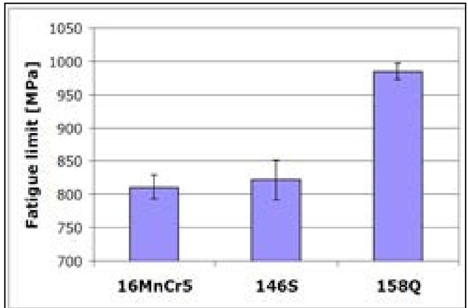
Figure 11 Fatigue limit for notched RBF samples; error bars show 95 percent confidence.
