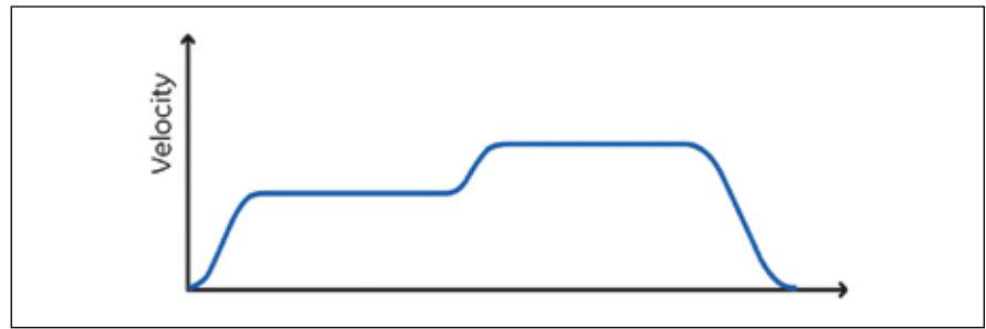
Figure 5—100% jerk control requires exactly twice the acceleration torque from the motor compared to linear acceleration in the same amount of time.
