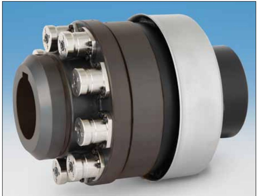
let. These safety couplings have four body sizes and anywhere from three to nine plungers, depending on torque setting. The adjustable plungers can be added or removed after installation in case of miscalculation of the torque value release. The ST is also available as a pure torque limiter or with integral gear coupling or disc coupling.
