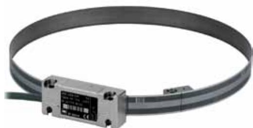
Depending on the shaft diameter, up to 20,000 line counts are available on the MSR 40. Each version offers quasi-absolute positioning via distance-coded reference marks or homing via a single reference mark. The encoder is available in standard and custom sizes.
