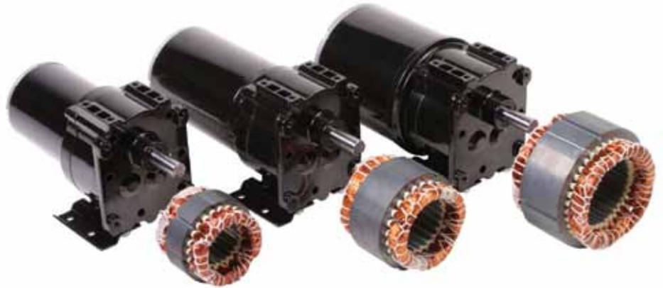
In response to trends for smaller OEM equipment with higher power output, the 100 mm AC motor line from Bison Gear and Engineering Corp. offers 1/8 horsepower in 30 percent less volume than previously available. The four inch diameter single phase motors have been mated to Bison's 750 Series right angle gearing to offer up to 104 inch-pounds (11.8 N-m) of continuous torque in a compact package with three-wire reversible hookup and a range of mechanical options.
