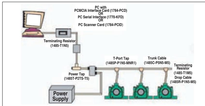
Figure 3—Condition monitoring system set-up (courtesy of Baldor-Dodge-Reliance).
