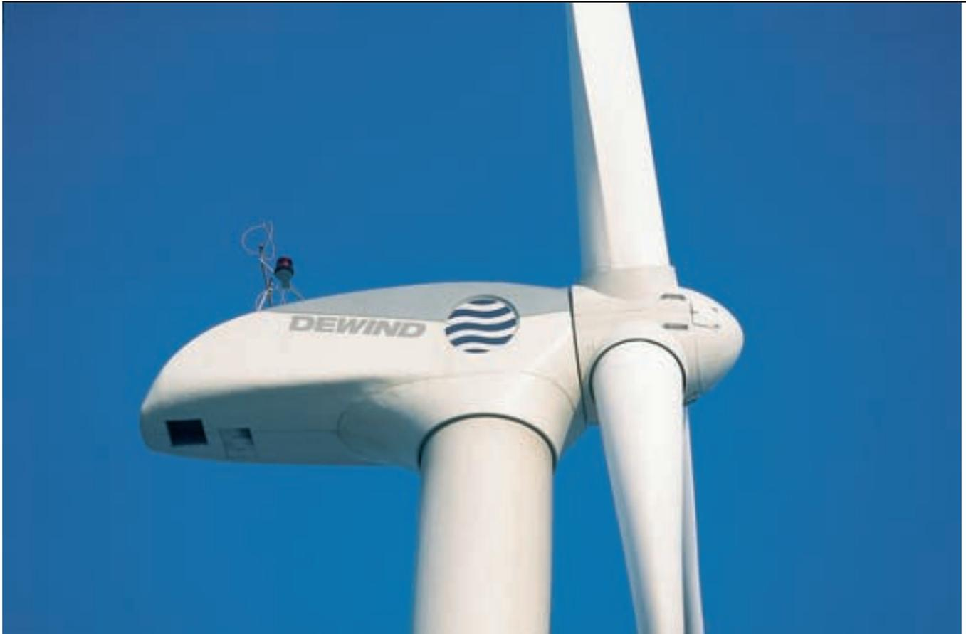
With Voith's WinDrive technology, the maximum operating loads in the drivetrain are reduced by up to 20 percent for the tower and foundation.
