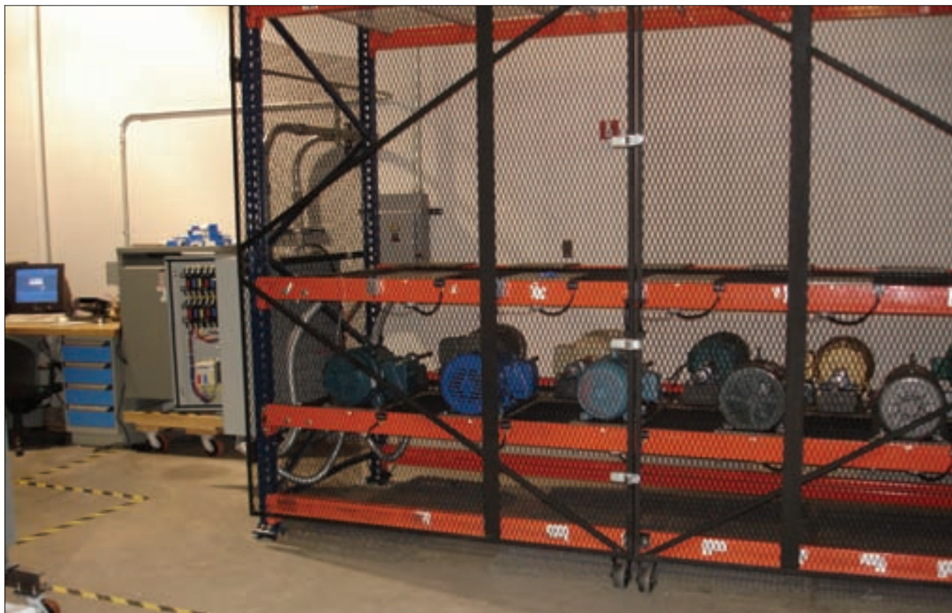
Motor reliability test bed.
