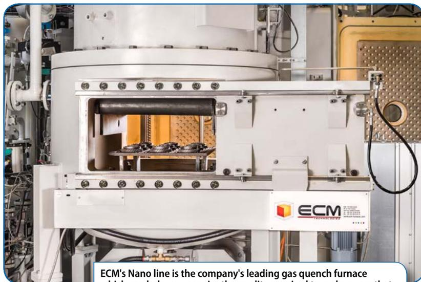
ECM's Nano line is the company's leading gas quench furnace which can help you acquire the quality required to make gears that will succeed in an electrified automobile.
