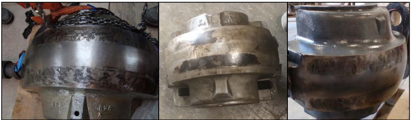
Figure 3 Three separate liners that have failed due to high fan vibration levels and show the fretting corrosion marks along their spherical seats.
