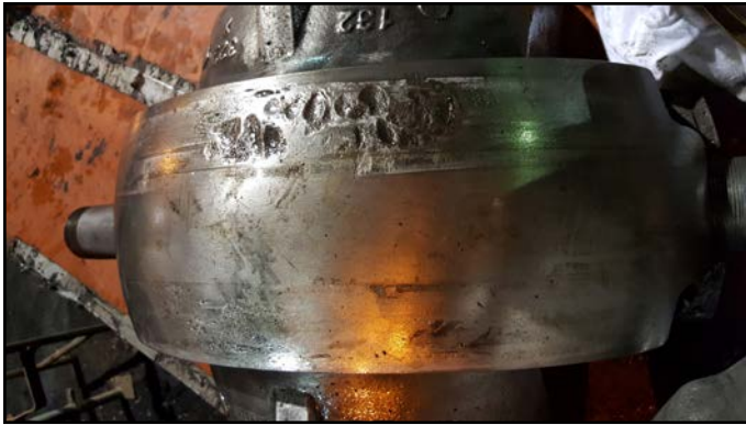
Figure 2 A new liner installed into an old housing failed after ~1 to 1½ years of operation and caused an unexpected fan shutdown due to high vibration levels. The deep pitting and fretting corrosion caused by improper seating of the liner in the housing can be clearly seen.
