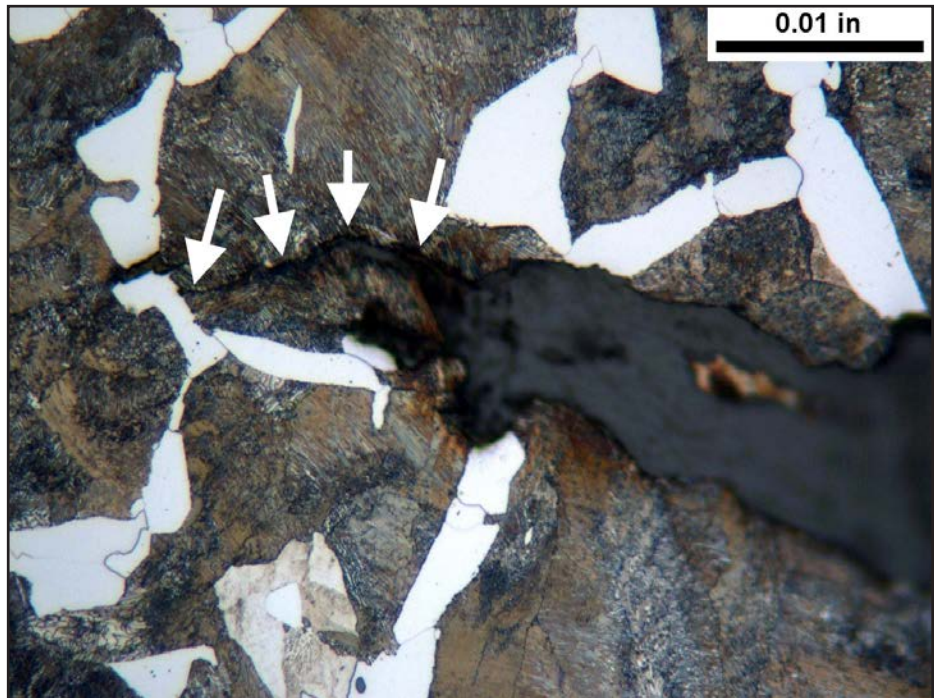
Figure 9 A higher magnification view of the right-center portion of Figure 8. Arrows indicate the presence of corrosion scale in tip of crack; 2% nital (OM 500x)
