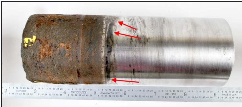
Figure 1 Fractured shaft, as received. Yellow marking indicates 12 o'clock position arbitrarily identified by Element New Berlin. Arrows indicate fretting damage.
