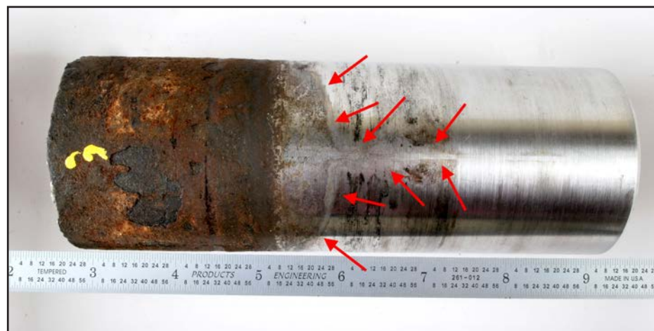
Figure 2 Three o'clock position of shaft after rotating piece 90°. Arrows indicate pattern of fretting damage. Pattern of fretting damage suggested non-uniform contact on bearing. Pattern at 3 o'clock position indicated region of non-contact when bearing was present.
