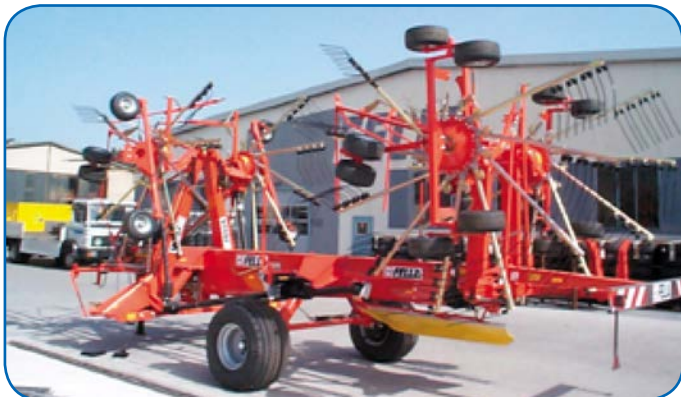
Figure 5 Spreaders. Main reasons for iglide bearings: The special design to complement the centrifugal arm results in a significant reduction of manufacturing costs. It is also maintenance-free and has high wear resistance (Fella Werke GmbH & Co. KG).
