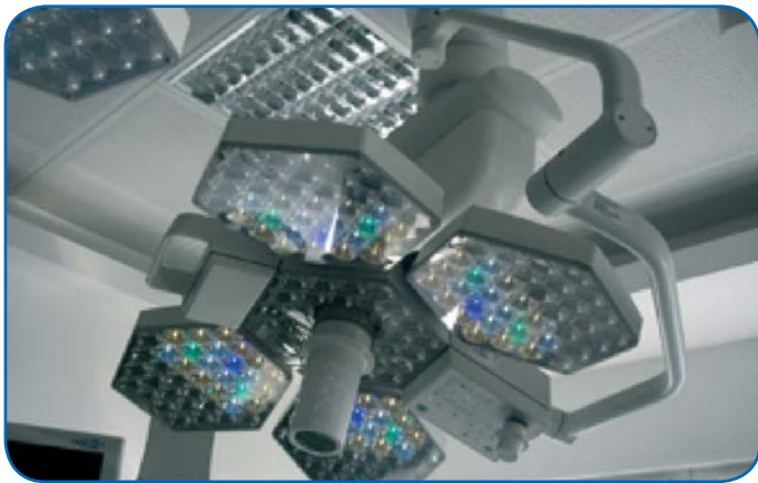
Figure 4 Surgical Light. The motor-powered swiveling LED wings are adjusted with the aid of iglide JVFM bearings. Self-lubricating and maintenance-free (Trumpf iLED Medical Systems Inc.).
