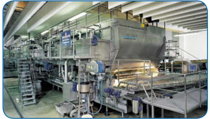
Figure 3 Washing chain bearings. Reduction of the drive power for bottle washing machines by using iglide under the most difficult conditions in a 2-3% caustic soda and temperature of +176°F (Krones AG).
