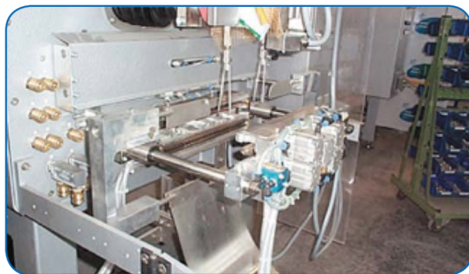
Figure 8 Tubular bag machines. The continuous operating temperature in the bonding arms frequently reach + 320°F and higher. These requirements are met by iglide Z bearings which also offer particularly high resistance to wear (Affeldt Verpackungsmaschinen GmbH).
