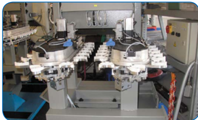
Figure 6 Tool changer chain. Main reasons for iglide bearings: Enormous cost advantages in comparison to standard metallic rolled bearings as well as low coefficient of friction and with soft shaft materials (Deckel Maho Seebach GmbH).
