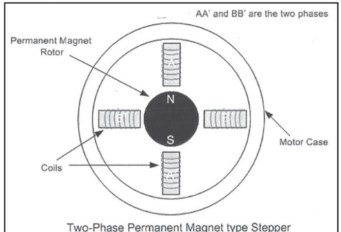
Figure 2 A two-pole rotor magnet and four stator teeth—each with a copper winding and an operating excitation sequence of A, B, A<sup>1</sup>, B<sup>1</sup>. There are some military and space applications that use this motor type with a rare earth rotor magnet.
