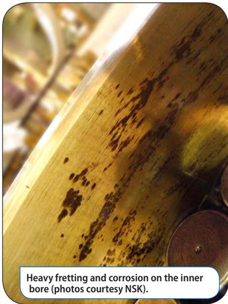
Heavy fretting and corrosion on the inner bore (photos courtesy NSK).
