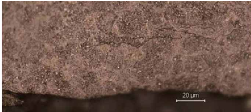
Figure 8—Severe wear damage phase under contaminated conditions.
