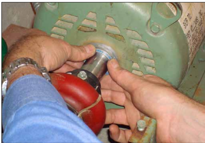
Figure 5—One hour after installation, epoxy has cured and motor again tested with oscilloscope and probe. Now—with VFD set at 60 Hz; motor running at 1,775 rpm (7.4 amperes); and oscilloscope set at 10 millivolts and 100 microseconds-per-division—discharge plot displayed on scope is essentially a straight line, indicating shaft voltage discharges were diverted by Aegis ring to ground.
