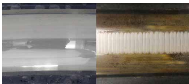
Figure 8—New bearing (left); fluted bearing (right).
