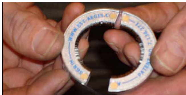
Figure 2—Equal proportions of epoxy and activator are mixed and small amounts are applied to the back of the ring.
