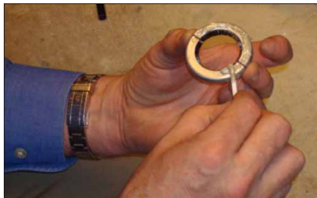
Figure 3—Narrow band of Aegis colloidal silver coating is then applied around the shaft to improve surface conductivity. Ring is then installed on the shaft and re-taped.
