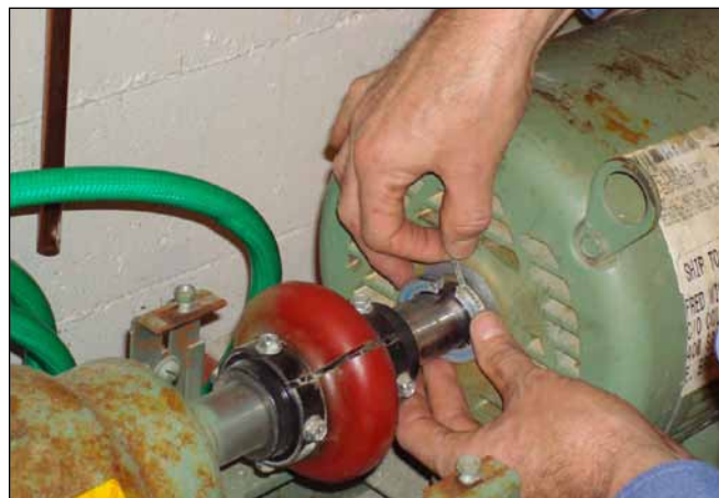
Figure 4—Ring is pushed back against bare metal of end-bracket, maximizing electrical contact via conductive epoxy. To ensure ring is correctly centered on shaft, metal spacers (included in the kit) are inserted into gaps between two halves of ring. Post adhesive cure, spacers are removed. Installation time: about 10 minutes.
