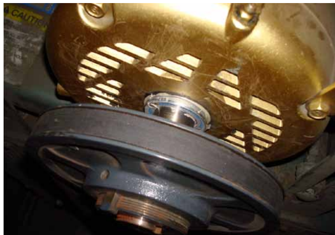
Figure 7—Hand-held heater is used to speed epoxy's cure; post-curing, shaft voltage is measured again, showing a reading of only 380 millivolts, peak-to-peak.
