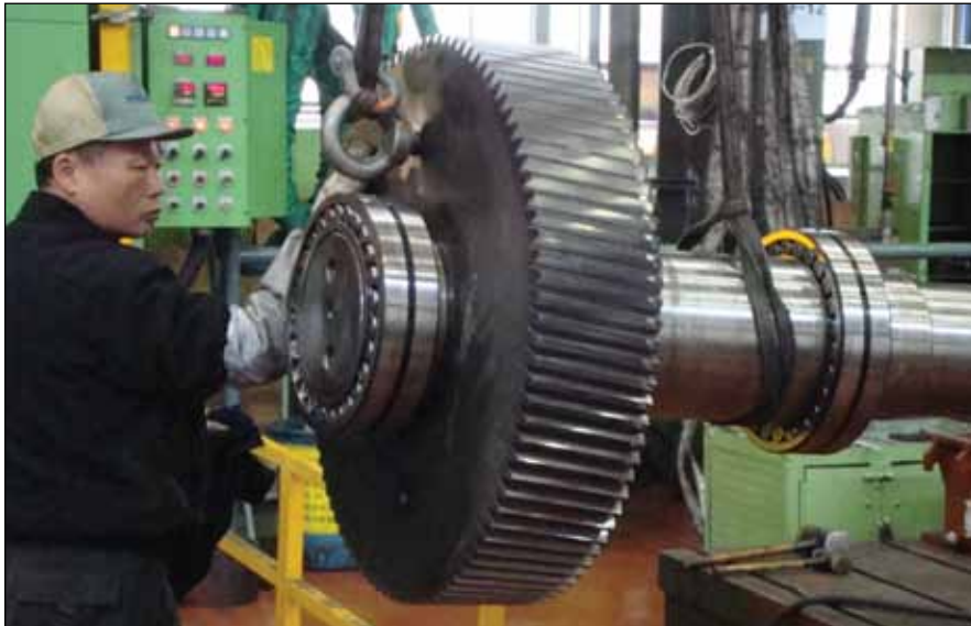
SKF CARB bearings allowed the Hyosung Corporation to downsize the gearbox for high sea operations (courtesy of SKF).
